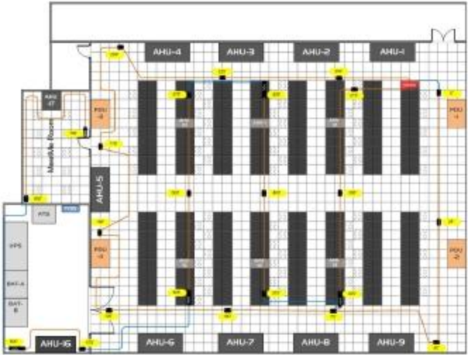
Uploaded reference map can be configured to display the location of the leak
